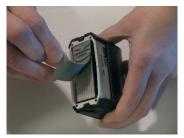
Peel the existing die off the device plate surface. Rubber die should remove easily. Discard die.
